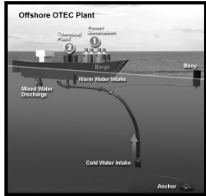
Fig.1: OTEC: Ocean thermal energy conversion, open and closed, [3].
