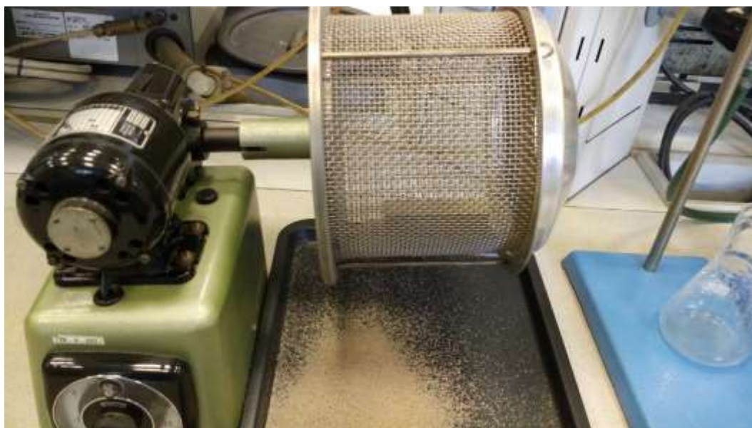
Figure 3 +GF+ device for measurement of abrasion resistance
