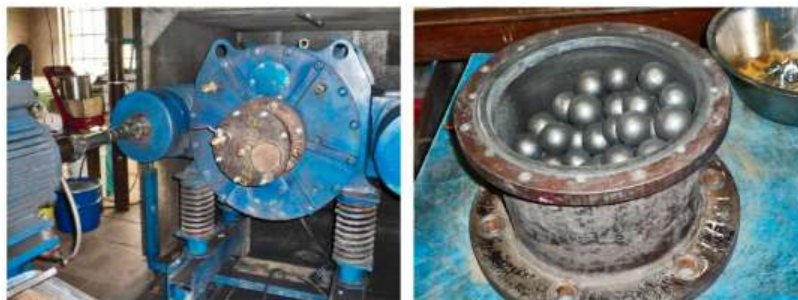
Figure 12 Eccentric vibratory mill with attached closed satellite (left), open satellite filled with balls (right)
