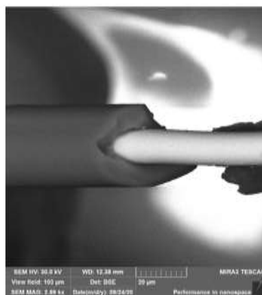
Fig. 2 SEM micrograph of typical \text{Ni}_2\text{FeGa} glass-coated microwire
